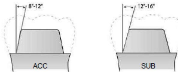
**Taper greater than 16 degrees is considered Critically Deficient.**
